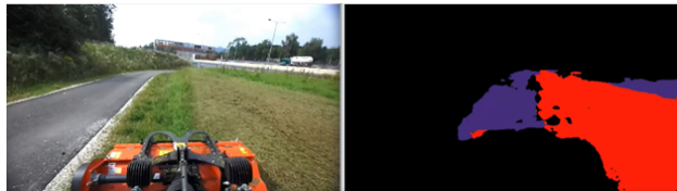
Figure 14. Smarter dataset: Segmentation of mown (red) and unmown (blue) meadows from the view of the tool carrier.
