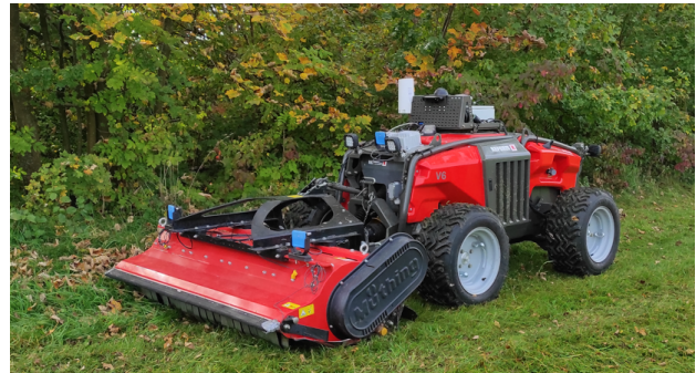
Figure 1. Metron P48RC is a radio-controlled tool carrier with a true hybrid drive.
