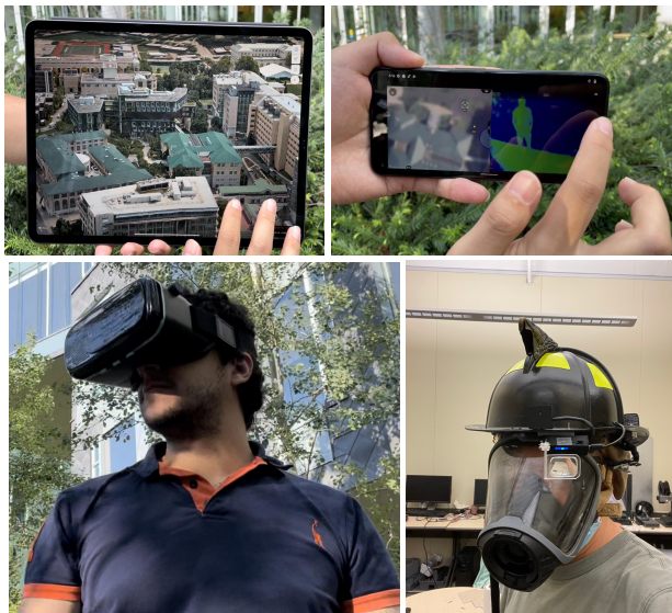
Figure 2. UI/UX design for improving the mobility of the incident command dashboard: 1) Dashboard on iPad and 2D/3D tablet Lume, 2) Dashboard on iPhone and Android phone, 3) Google Cardboard-based stereo display, and 4) the holographic dashboard on first responder's helmet.
