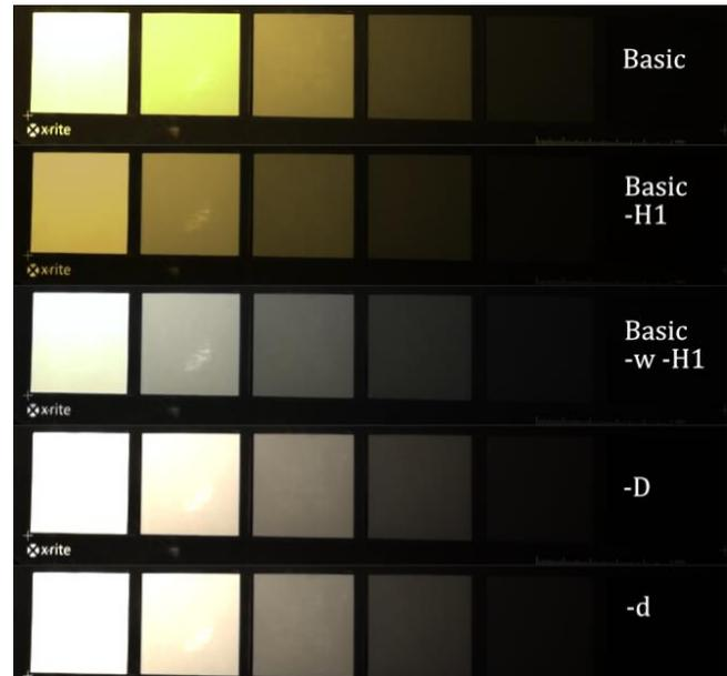
Figure 5. Color cast of the neutral ColorChecker24 patches for the CIE F12 image
