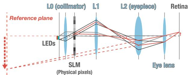
**Figure 2.** An optically equivalent model of the LF display test bed. Light beam(s) for a single viewpoint and a single pixel is shown. Black and gray lines indicate marginal light from the light source responsible for the viewpoint. Red lines indicate the light for imaging the pixel on the retina.
