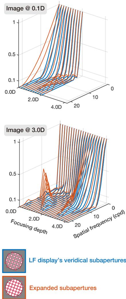
**Figure 7.** Simulated SFRs for the LF display model (blue curves) and for a hypothetical display model with expanded subapertures (red curves). As examples, the responses for images rendered at 0.1 and 3.0 diopters are plotted in the same manner as in Fig. 4.
