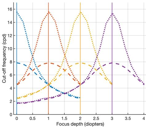
**Figure 8.** Cut-off frequencies for the gain of 0.1 in the SFRs simulated in the original display model (dashed lines) and the hypothetical display model with expanded subapertures (dotted lines).
