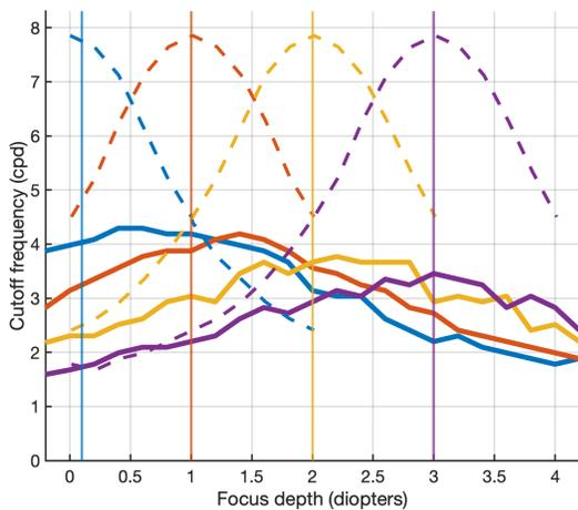
**Figure 5.** Cut-off frequencies for the gain of 0.1 in the SFRs as functions of camera's focusing depth. Blue, red, yellow, and purple curves are the cut-off frequencies for the image depths of 0.1, 1.0, 2.0, and 3.0 diopters, respectively; the image depths are also shown as vertical lines with corresponding colors. Solid and dashed curves correspondingly indicate the measured and the simulated results.
