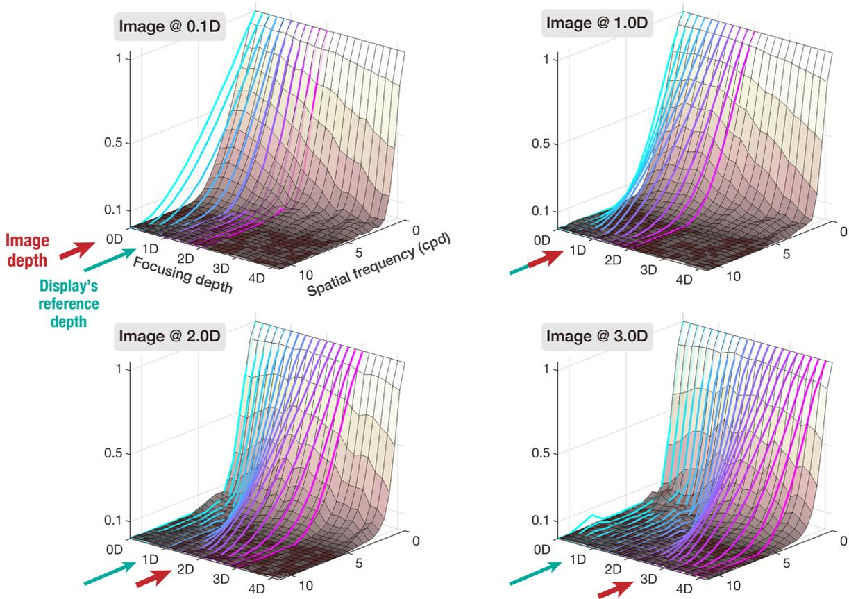
**Figure 4.** Measured and simulated spatial frequency responses (SFRs) about images rendered at 0.1, 1.0, 2.0, and 3.0 diopters. 3D surfaces and colored curves indicate the measured and simulated SFRs, respectively. The SFRs, which are functions of spatial frequency, are visually stacked over the camera's focusing depth, and the image depth and the display's optical reference plane depth are respectively shown by red and green arrows.
