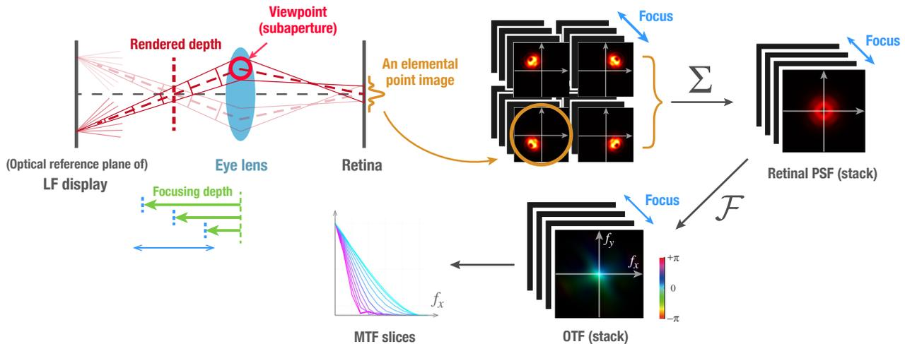
**Figure 3.** The model of an LF display and the process of simulation and evaluation of rendered retinal images. An LF display that renders a point with four beams is modeled, but only two beams are shown in the diagram for simplicity.
