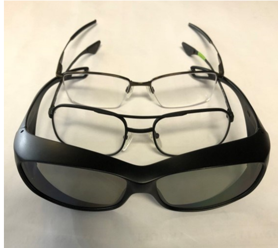
Figure 5. Stacked eyewear used in eyewear study: 1) Circular polarizing 3D glasses; 2) + 0.5 D optical add in aircrew-approved frames; 3) operator’s prescription eyewear.
