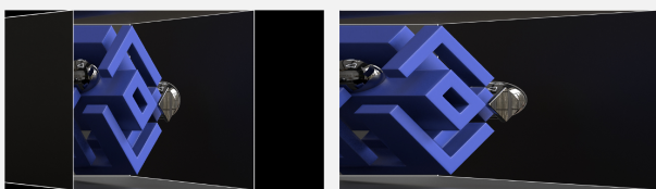
Figure 10: Object rendered without distortion map (left) and with distortion map (right).
