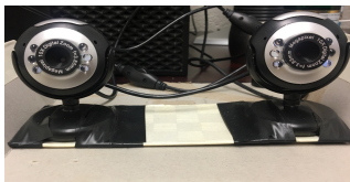
Figure 1: A basic stereo imaging setup was created. The prototype is comprised of two USB webcam cameras with a 3.85mm 10x focal length, and were positioned six inches apart from each other.
