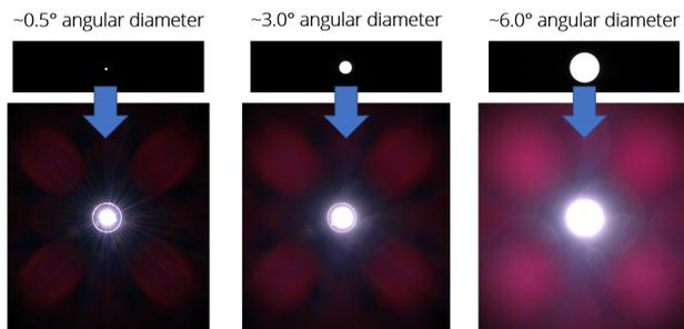
**Figure 10.** Example showing the effect of light source angular diameter on the appearance of stray light. The cropped images on top were well-exposed to show the actual size of the source in the image without any blooming. The cropped images beneath were captured with longer exposure to reveal stray light. The halo surrounding the direct image of the source is caused by reflections from within the light source collimator.
