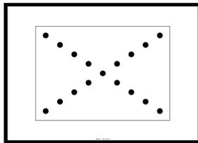
**Figure 3.** An example of an Imatest-branded backside-illuminated chart design that could be used for the patch-based approach to stray light testing. The design is meant to be compliant with ISO 18844:2017.
