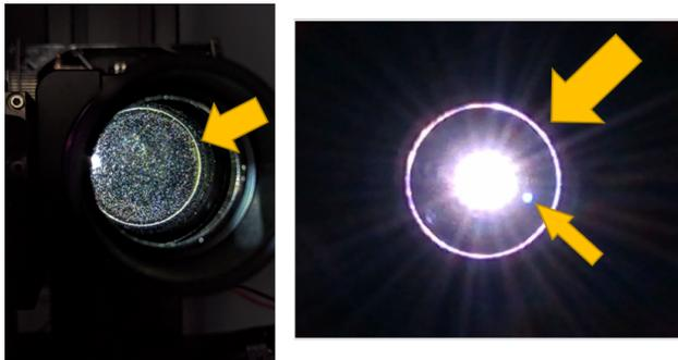
**Figure 8.** Example images showing how extraneous reflections from inside a refractive collimator (left) can show up as stray light in the image under test (right). In the latter image (which is significantly cropped), a halo surrounds the direct image of the source – a result of extraneous reflections inside the collimator. In addition, dust and smudges on the collimating lens surface can appear surrounding the direct image of the source.
