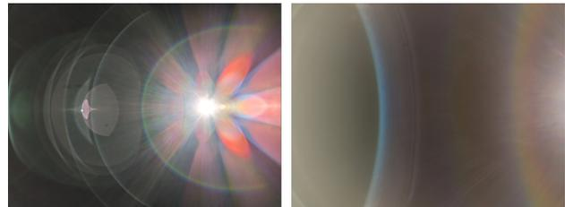
Figure 1. Two examples of test images showing stray light manifesting itself in different forms. The left image shows a small, bright light source within the camera FOV resulting in clear examples of petal flare and other ghost artifacts. The right image shows significant veiling glare and other artifacts caused by a small, bright light source outside the FOV of the camera. Both images were captured in a completely dark lab using a Google Pixel 6 Pro camera.
