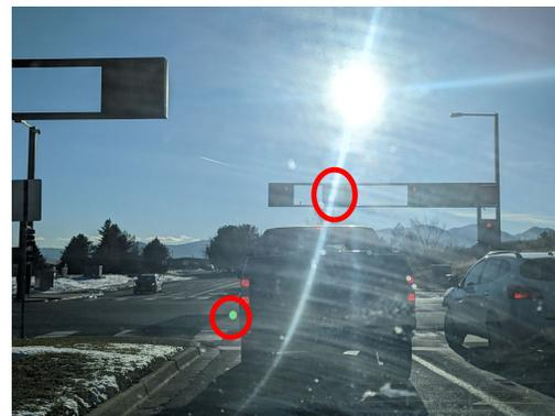
Figure 2. An image of a traffic intersection captured through a windshield using a Google Pixel 6 Pro camera. Stray light artifacts emanating from the Sun obstruct the view of the traffic light. Some of these artifacts are caused by the windshield. Separately, some stray light caused by the camera is manifested as a ghost in the form of a peculiar green dot.
