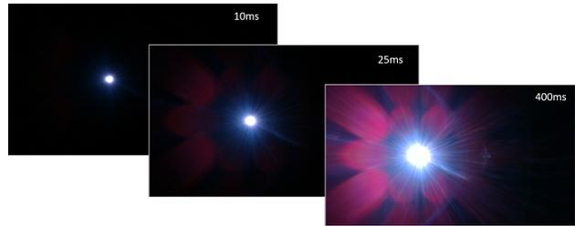
**Figure 7.** Three images captured with the same camera using different integration time to show different levels of stray light. In the rightmost image which was captured using the longest integration time, fainter levels of stray light are revealed, but the ability to measure stray light close to the direct image of the source is limited due to saturation and significant blooming.
