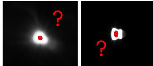
**Figure 6.** Two cropped images of a small, bright light source demonstrating that the shape, size, and location of the direct image of the source may be ambiguous. The ambiguity can be caused by lens distortion, blooming, coma, and stray light. The red ellipsoids illustrate the question of where and what the actual direct image of the source is (and the overarching question of what is stray light).
