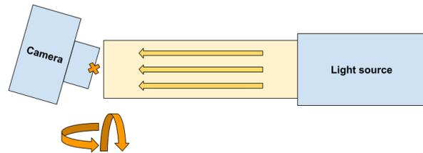
**Figure 4.** High level diagram of the small, bright light source approach. The light source projects a small, point-like source as a collimated beam of light that overfills the front of the DUT. The DUT is rotated (or the source moved) to change the angle of the light source with respect to the DUT. The DUT is rotated about its front to avoid inducing a lever arm, minimizing the necessary area of the projected beam.
