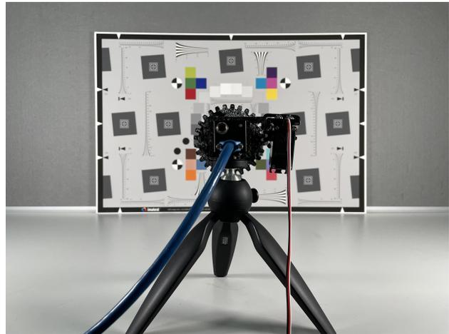
**Figure 2.** Test setup for through focus sweep.
