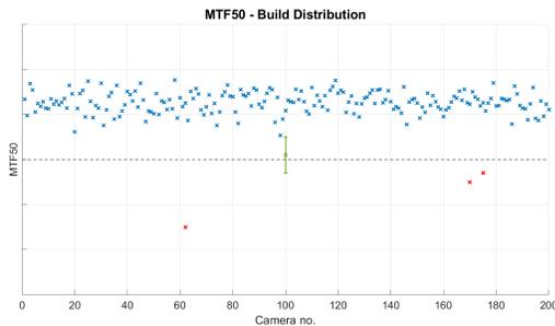
**Figure 1.** Exemplory distribution of camera MTF<sub>50</sub> measurements at end of line testing. Pass/fail limit is indicated by the dashed line
