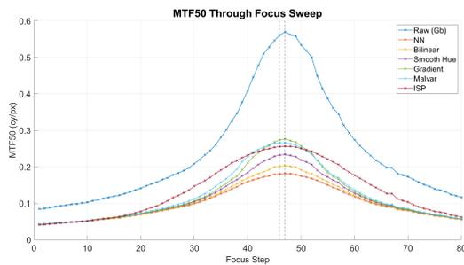
Figure 6. MTF50 measurements during through focus sweep
