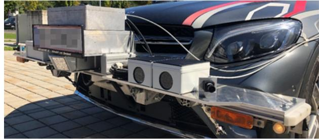
Figure 1: Sensors are mounted for the purpose of prototyping on an easily accessible rail in front of the car.
