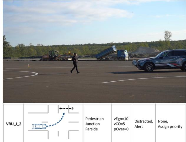
Figure 5: Video recording and scenarios description of interaction between pedestrian and vehicle on an automotive proving ground.
