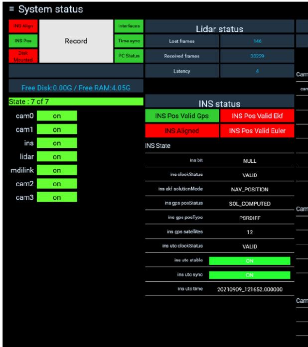
Figure 4: The human computer interface allows for control and supervision of the recording system. Free disk space, mounted disks, free RAM and the INS status as well as successful connection to the sensors are supervised during recording.
