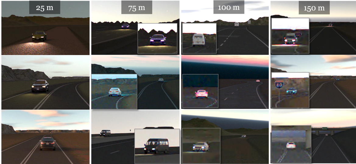
Figure 2. Examples from the scene collection for assessing spatial resolution. Each column shows three of the 50 scenes comprising a randomly selected car on a rural road. In some of the images we use an inset to render the car. The scenes can be rendered under different illumination conditions, day to dusk are illustrated. We did not include streetlights in this collection.
