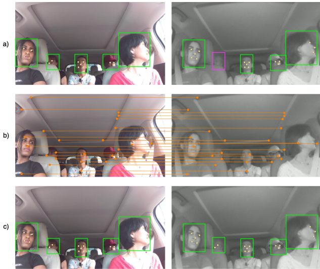
Figure 7: Fixing annotations across different camera modalities and illumination conditions; a) shows the offset between the camera modalities and a missing face annotation in the IR stream. b) shows the LoFTR keypoints used to estimate a homography to align the annotations. c) shows a consistent set of annotations suitable for both the camera modalities and lighting conditions.
