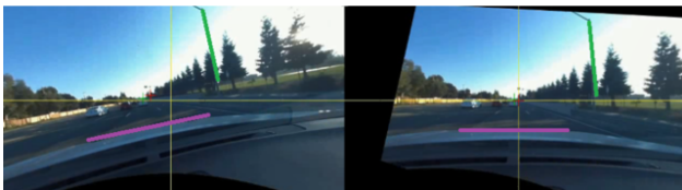
Figure 10. Left: hand labelled horizontal (purple) and vertical (green) line segments. Right: labelled horizontal (purple) and vertical (green) line segments after roll angle correction.
