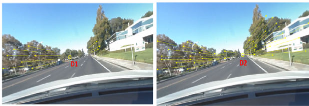
Figure 3. tRANSAC example 1. Left: RANSAC estimation of lane vanishing point (D1) by optical flow features extracted from single frame. Right: tRANSAC estimation of lane vanishing point (D2) by optical flow features accumulated dynamically across time. (only inlier optical flow vectors are shown for better visualization.)
