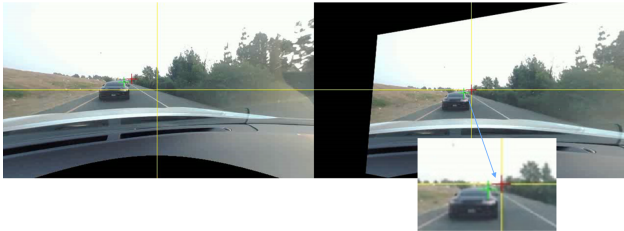
Figure 9. Warped vanishing point (VP) error. Top left: red color cross - estimated vanishing point, green color cross - hand labelled vanishing point. Top right: image after warping estimated vanishing point to image center. Bottom right: warped vanishing point (VP) error is defined as distance between labelled vanishing point (green color cross) and estimated vanishing point (red color cross) in warped image in which estimated vanishing point lies in image center.
