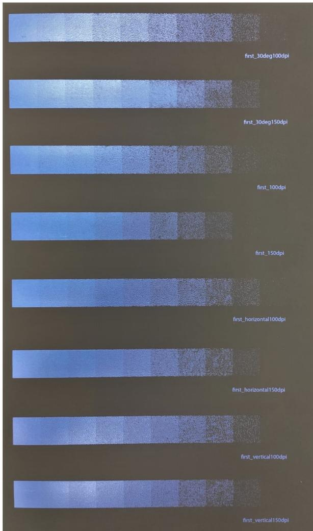
**Figure 3.** Example of a set of printed wedges with increments of 10 per cent in intensity, halftoned at 100 dpi and 150 dpi. In descending order the image shows: First-order halftoning where the structure is aligned at 30°, symmetrical first-order FM, horizontal alignment and vertical alignment with regards to x-axis.
