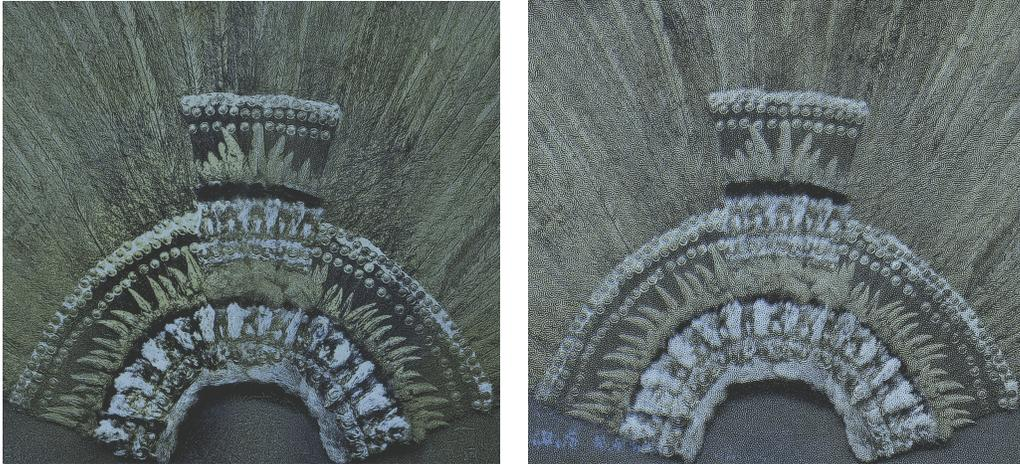
**Figure 4.** Details of prints with green and blue layers made with structure-aware halftoning (left) and second-order FM halftoning (right).
