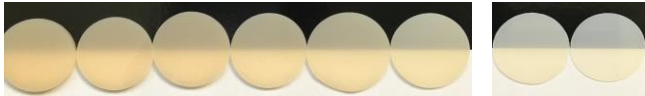
Figure 1: Samples of the Estelite Universal Flow Medium material shade A2 on a drawdown card (no optical contact). The picture is taken in daylight with an uncalibrated camera. Samples are sorted from the thickest on the left to the thinnest on the right: 2.0 mm, 1.6 mm, 1.5 mm, 1.2 mm, 1.0 mm, 0.8 mm, 0.5 mm and 0.4 mm.
