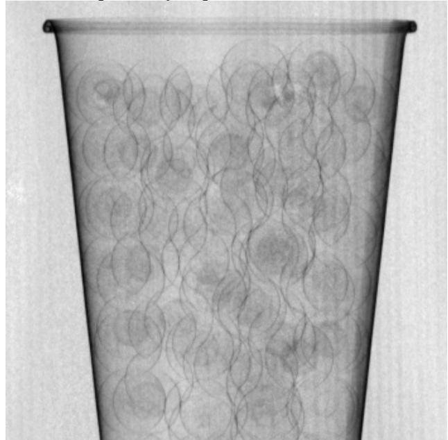
Figure 1: Example dark field image of wax paper cup filled with plastic spheres. The sample appears nearly edge detected, which is poor match for regularization techniques such as total variation.
