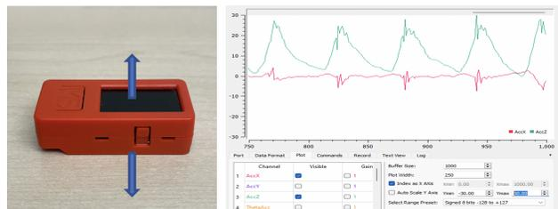
Figure 6. Acceleration is perpendicular to the ground along the  $Z$ -axis (in green)
