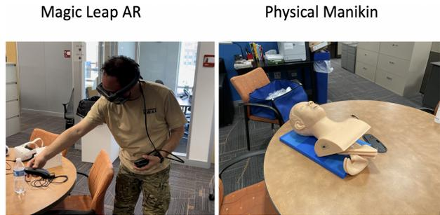
Figure 15. Integrating an AR headset with a physical manikin enables VR object overlay and haptic feedback.
