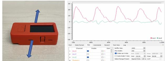
Figure 5. Acceleration is parallel to the ground along the  $X$ -axis (in red).
