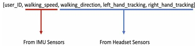
Figure 3. A fused data string from the IMU sensor and the headset
