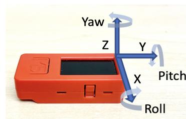
Figure 1. The 6-DOF IMU sensors with accelerometers and gyroscopes
