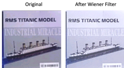
Figure 10. The original digitally zoomed image (left) and after Wiener Filter (right)
