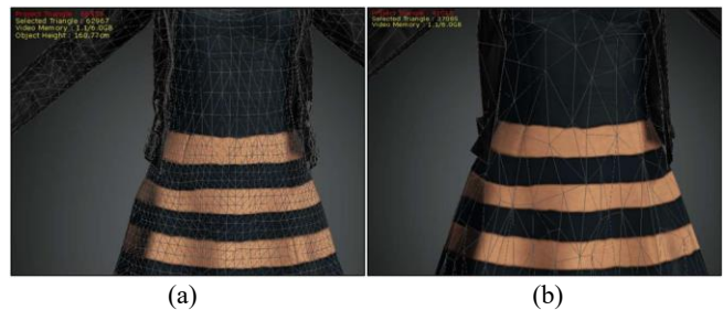
Figure 9. Illustrations of utilized Insta LOD polygon reduction approach for optimization of virtual characters. (a) 62,967 triangles Initially on a virtual character without polygon reduction with Insta LOD feature applied and (b) 37,085 triangles Initially on a virtual character with polygon reduction with Insta LOD feature applied.
