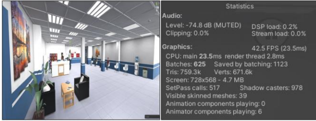
Figure 10. Illustration of a game instance (i.e., clinic visit scene in Charles's case) without the utilization of occlusion culling optimization technique.
