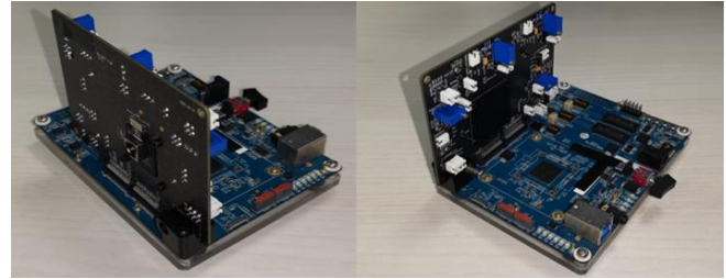
Figure 6. Test Zig Board for getting raw data of image sensor
