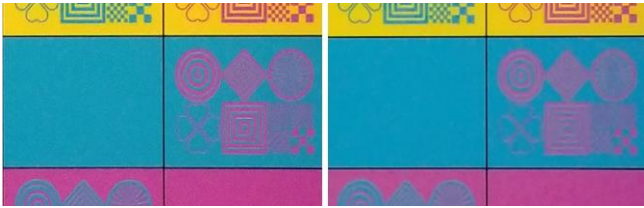
Figure 10. Image Quality, Detail Loss: (a) RGB Sensor, (b) CMY Sensor
