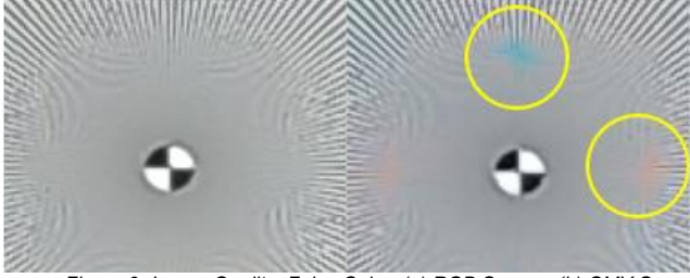
Figure 9. Image Quality, False Color: (a) RGB Sensor, (b) CMY Sensor
