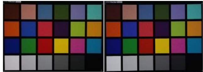
Figure 13. IQ, Color Accuracy of Low Lux: (a) RGB Sensor \Delta E_{ab} 9.3, (b) CMY Sensor \Delta E_{ab} 10.74, Chroma Noise (a) 1.57, (b) 2
