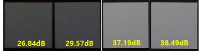
Figure 12. IQ, Y SNR of Low Lux: (a) RGB Sensor 26.84dB, (b) CMY Sensor 29.57dB, indoor (a) 37.19dB (b) 38.49dB
