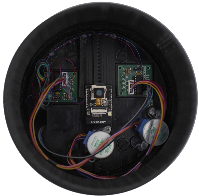
Figure 10. Inside Lafodis: electronics and Herringbone gear drive
