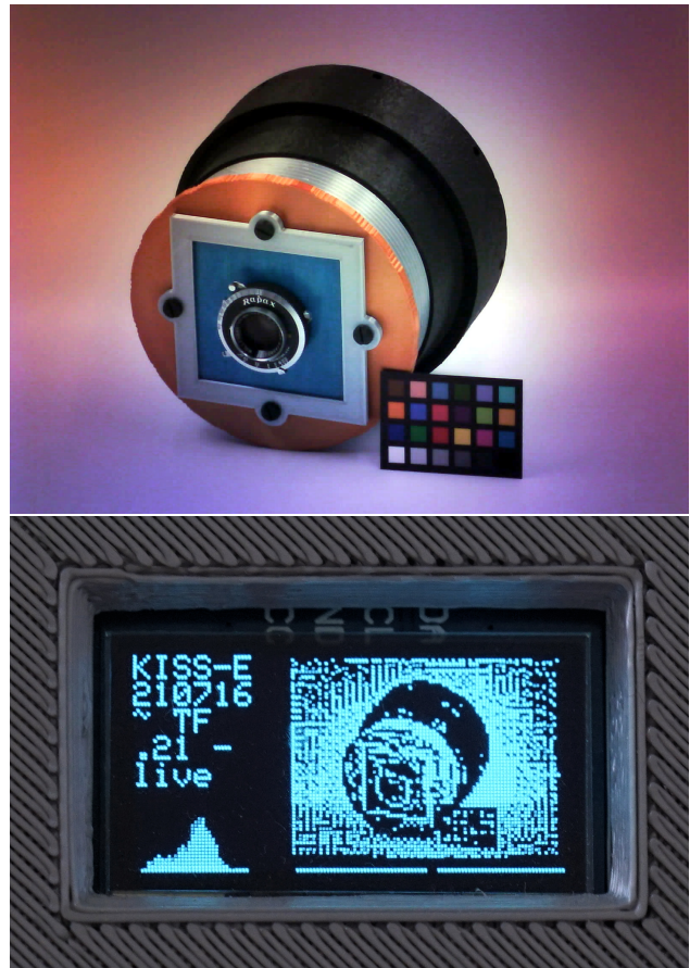
Figure 7. KISS-E capture of Lafodis and corresponding OLED live view
