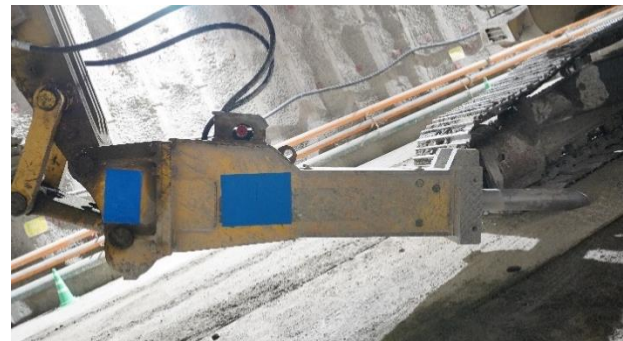
Figure. 1 Installation example of markers
