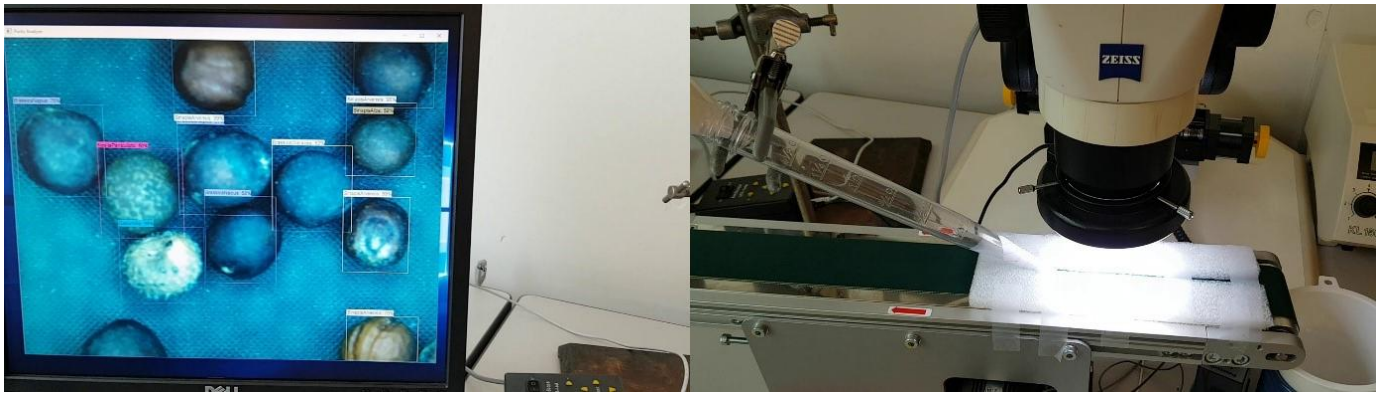
Fig. 3. Prototype of a Purity Analyzer System. Software (illustrated left) includes a CNN, called the Analyzer network, for object detection and classification. Another CNN, called the Detector network (not shown), facilitates training, validation, and testing. Hardware (illustrated right) comprises a seed container (not shown), a custom dispenser, a mini conveyor, an optical microscope, a ring illuminator, a digital camera, and a desktop computer (not shown).
