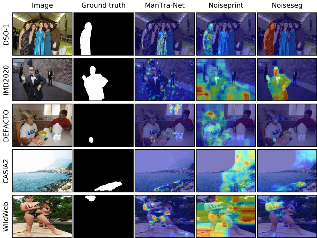
Figure 5. Examples from all datasets for NoiseSeg and the relevant baseline methods. From left to right: Spliced image, the corresponding ground truth mask, heatmaps of the predictions results overlaid on the spliced image for ManTra-Net, Noiseprint and NoiseSeg. On the heatmaps the color red indicates a high confidence that the region is spliced while blue indicates that it is pristine.
