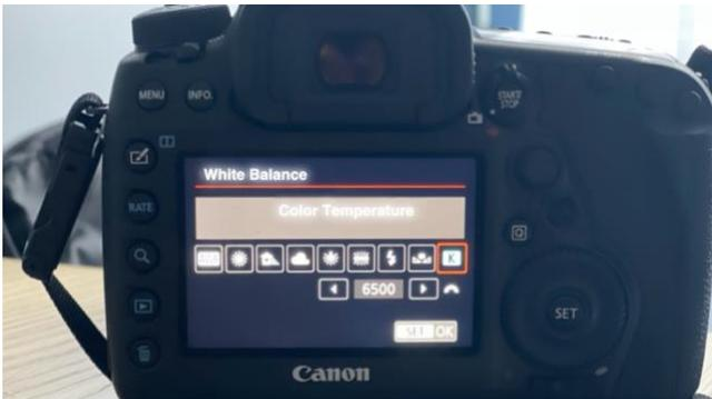
Figure 3. Color Temperature settings for Canon EOS D5 Mark IV camera [9]
