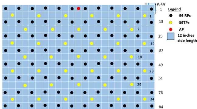
Figure 1: Hallway Layout for the Data Collection
