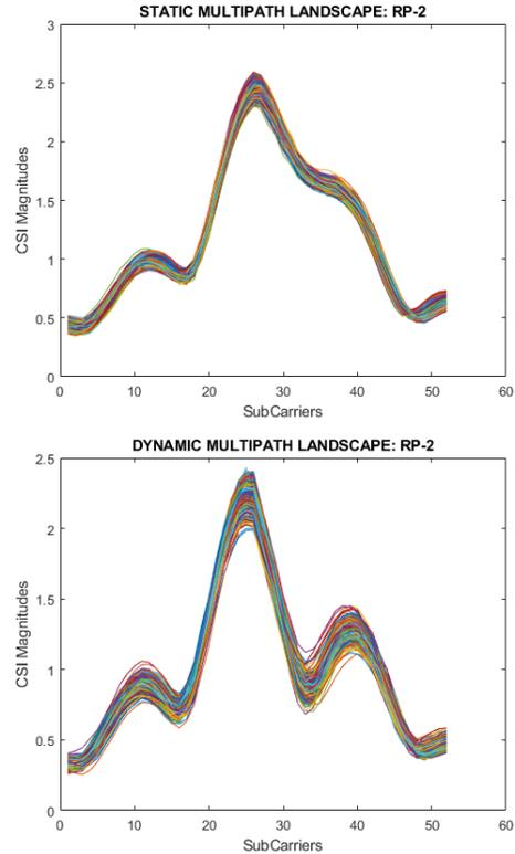
Figure 2: CSI plots of RP-2 at different multipath scenarios
