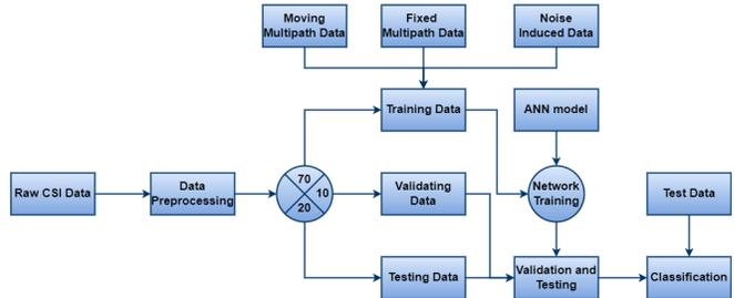
Figure 5: Block Diagram of ANN based CSI classification
