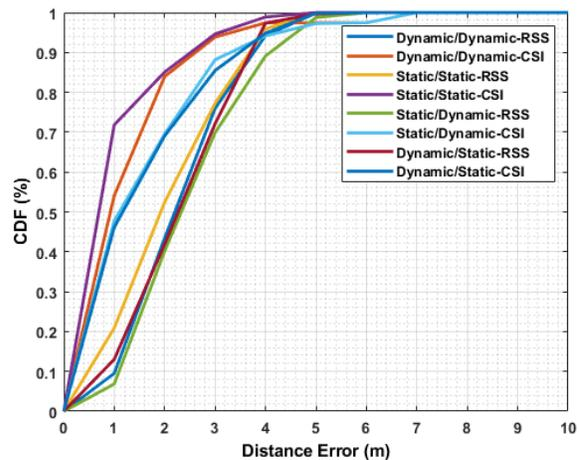
Figure 6: RSS vs CSI CDF plot of different multipath scenarios
