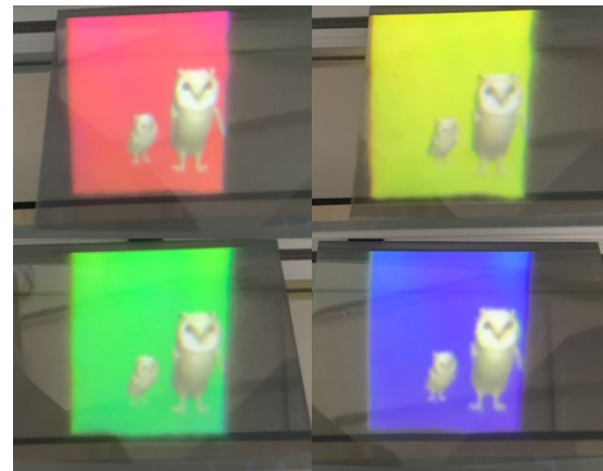
Figure 8. Spectroscopic experimental results of a naked-eye 3D display imaged in the air.
