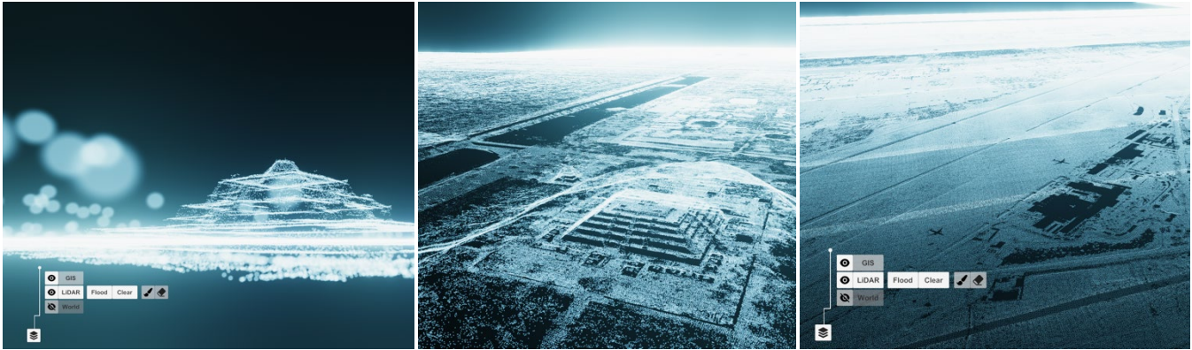
Figure 3. The LiDAR point cloud viewed from three different vantage points. Left: individual points are visible up close with the Baphuon temple present in the distance. Middle: the mountain temple of Phnom Bakheng in front of the moat of Angkor Thom. Right: the imprint of modern infrastructure can be seen as holes in the point cloud around Siem Reap airport.
