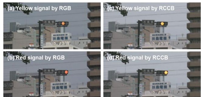
Figure 2. Yellow / Red traffic signal detection by RGB camera and RCCB camera.
