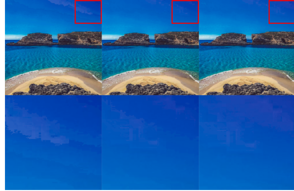
Figure 11. Simulated gamut mapping results illustrating the need for the blending-in steps. Left: GMA with naive gamut alignment, middle: GMA with gamut alignment & hue slice blending-in but without altitude bin blending-in, right: GMA with all the blending-ins.
