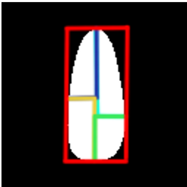
Figure 5: Results from Nail Mask Segmentation. Red bounding box gives an outline of the whole nail mask. The first, second, third and fourth quadrant are the areas bounded by the different color lines.
