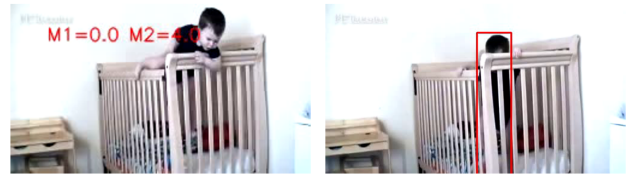
Figure 5. The two images are video frames of a sample output video. (left) M1 displayed in the video frame shows the value of M_B indicating the motion level of the background area. M2 displayed in the video frame shows the value of M_O indicating the motion level of the foreground area. (right) The output bounding box is shown in the video frame when the overall motion level is equal or greater than 5.
