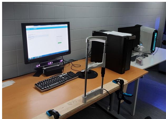
Figure 5: The setup used for the experiment. A stationary eye tracking device is installed below the monitor. The distance between the chin rest and the monitor is 60cm.
