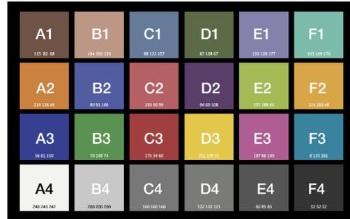
Fig 1. The target Calibrite ColorChecker Classic.
