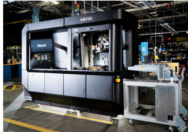
Figure 1. Xerox ElemX Printer 3D Aluminum Alloy Printer
