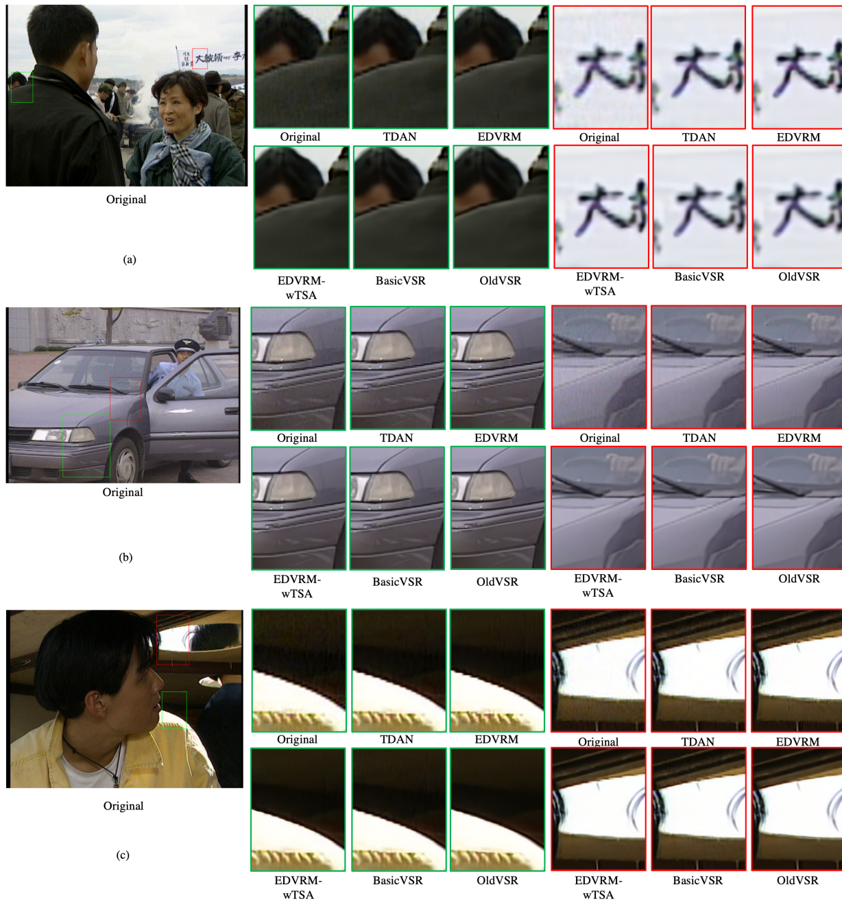
Figure 4. Qualitative comparisons (a) OldVSR restores correctly men's shoulder line. OldVSR and TDAN restores the letter (b) OldVSR restores correctly the pattern of the bumper and the edge of the bonnet. (c) OldVSR restores restores correctly the men's shoulder line and the edges of the round hole.
