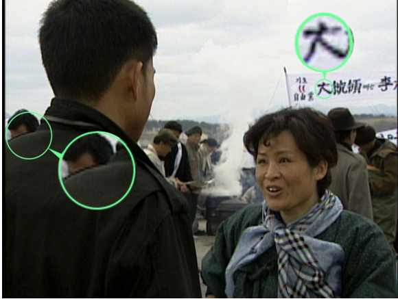
Figure 1. An illustration of visual artifacts found in old TV series. In this example, the deinterlacing and compression artifacts manifests as a stair pattern in the man's back shoulder. On the letter, we observe a comb-teeth pattern.
