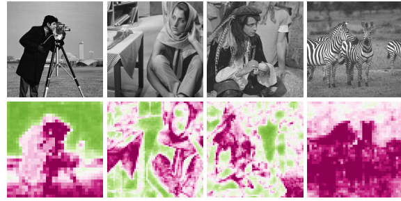
Figure 4: Visualization of the confidence maps for noisy images ( \sigma = 25 ). The threshold is 0.95 for better visualization, and all the values above it are green, while those below it are purple. The color intensity represents the distance to the threshold. The confidence map is 8 times smaller than the input stack.
