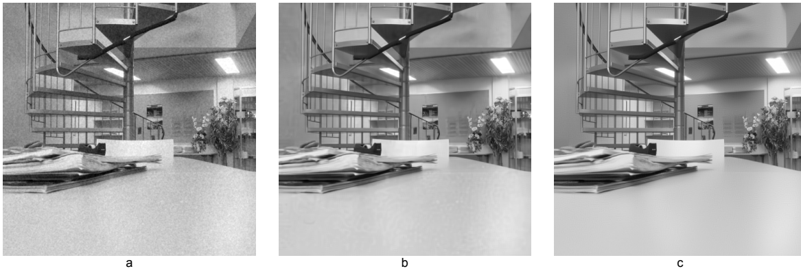
Fig. 7. Example of spatially correlated noise suppression: a) noisy image \sigma_b=0.8 , \sigma=5 , PSNR=34.2 dB, b) DRUNet+NLNet, PSNR=39.1 dB, c) DRUNet+PIXPNet, PSNR=39.2 dB
