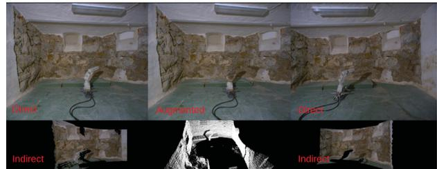
Figure 2: AROSS interface layout with all views enabled in Exp 1. In the left and right top row, two Direct camera views are shown, the top center view is a Disocclusion Augmentation view, in the left and right bottom row two Novel Perspective views are shown, and the bottom center view is a pure Lidar geometry view.
