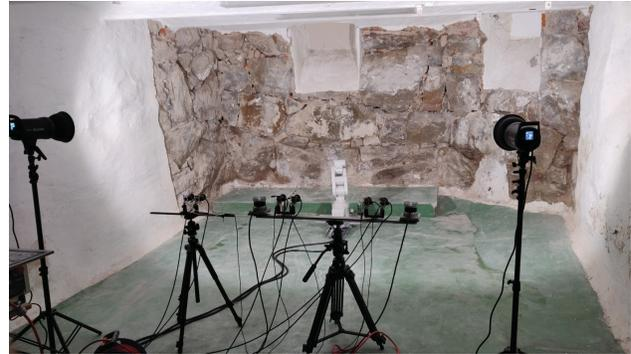
Figure 1: AROSS test set-up, with cameras, lights, remotely controlled robot arm, and the mine-like rock wall.
