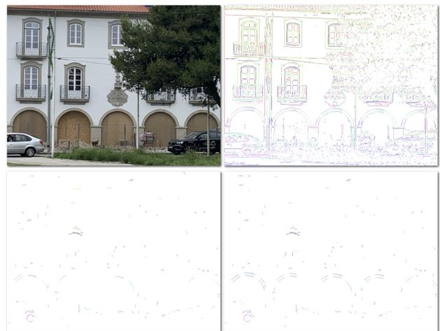
**Figure 8.** Circle detection example. Upper right, an edge-segmented image; below left, segments below threshold; below right, segments after merging.
