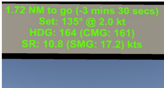
Figure 8: The Passage Manager provides the NavO with information on the distance to go to the end of the navigation passage, the current tidal set, the current speed made good and the speed required in order to arrive on time.
