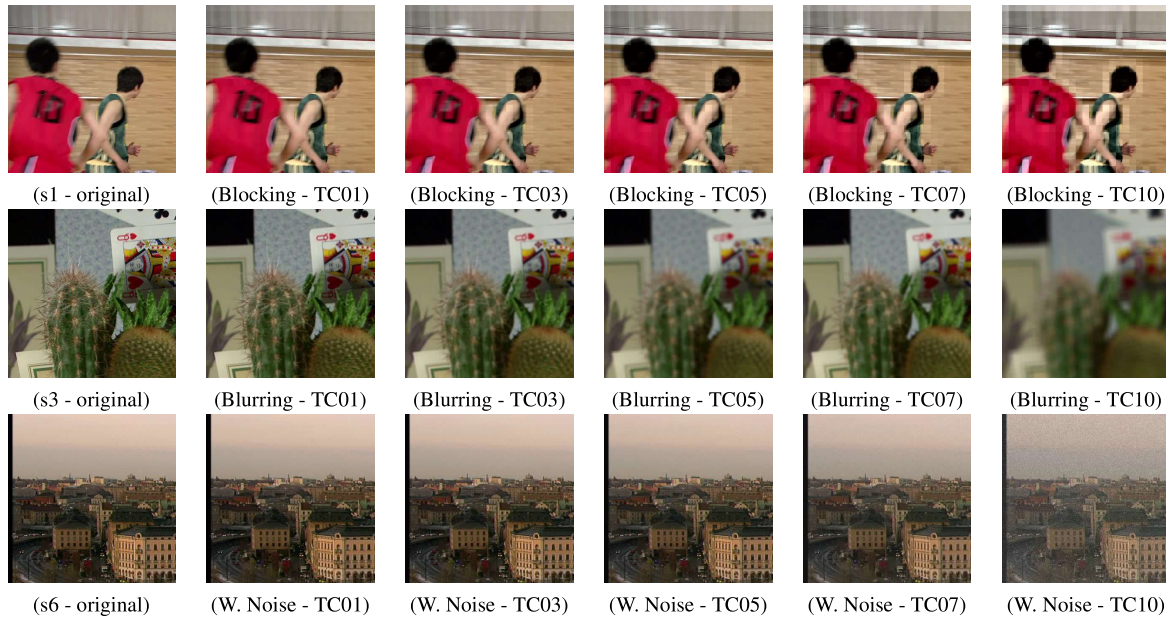
Figure 2: Sample frames of test videos of the Synthetic Database containing Blocking, Blurring, White Noise degradations with different levels of distortion (TC01, TC03, TC05, TC07, TC10).
