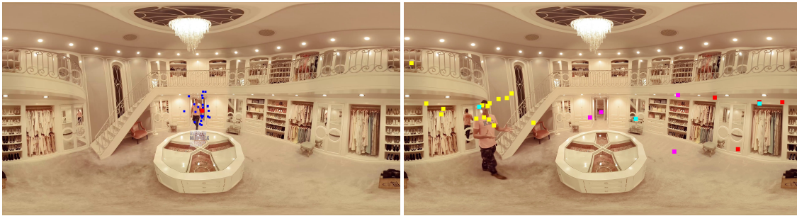
Figure 2: Two frames of a sample 360-degree video. The user data in the 1st frame (left) can be grouped in a single cluster, while the user data of the other frame (right) requires multiple clusters.
