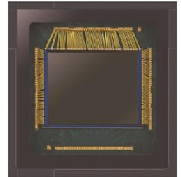
Figure 9. Die image of 108Mp CMOS image sensor
