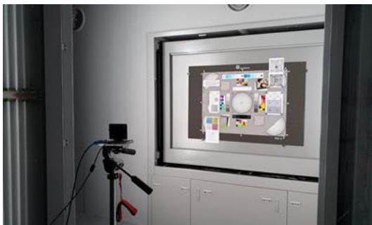
Figure 6. The proposed system uses a customized TE42 chart. This chart measures the various types of image quality with single capture.
