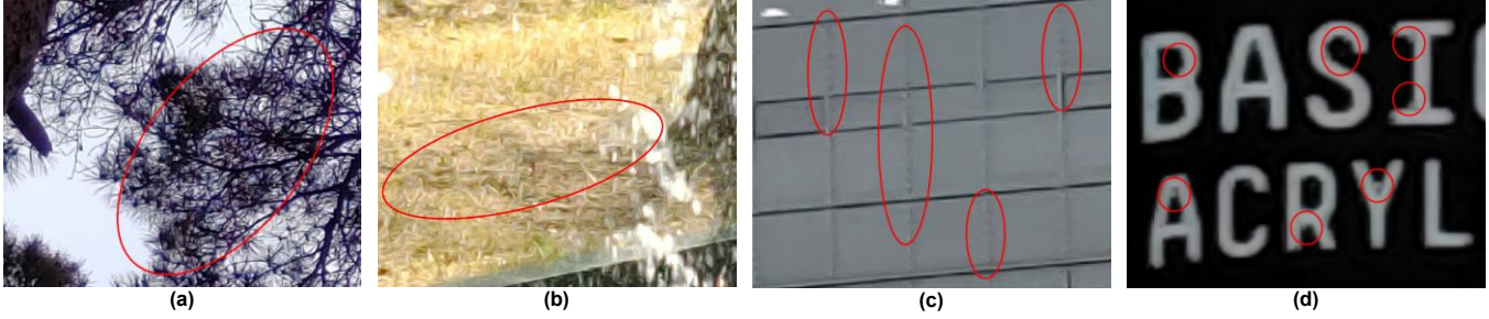
Figure 3. Example of remosaic artifacts: (a) false color, (b) color desaturation, (c) line broken, (d) corner dots
