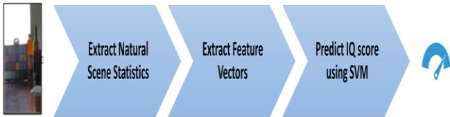
Figure 5. Block diagram showing evaluation of subjective image quality metric BRISQUE
