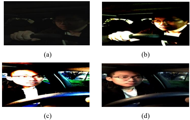
Figure 5: (a) Original dark image, (b) Dark image after applying histogram equalization, (c) Original extremely bright image, (d) Extremely bright image after applying histogram equalization
