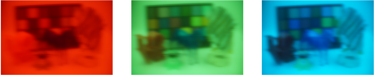
Figure 8. Sample scene captured through front-mounted color LCD with pixels set red, green, and blue
