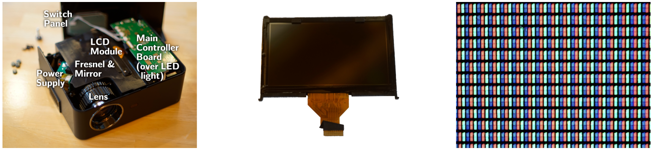
Figure 6. Inside the WiMiUS S2 mini projector, the extracted transmissive color LCD panel, and magnified backlit view of the LCD matrix
