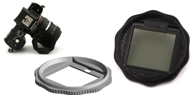
Figure 2. LCLV set in 3D-printed 55mm filter, model and as built
