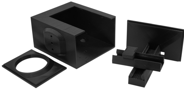
Figure 8. 3D-printed body parts of Lafodis 4x5
