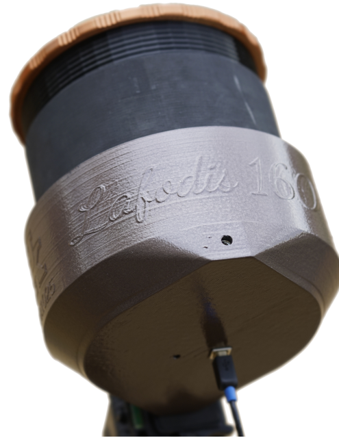
Figure 5. Lafodis160 LED power light and USB power cord
