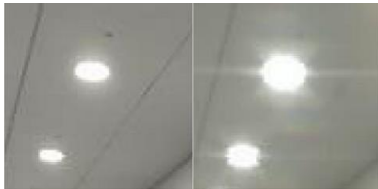
Figure 10. Image flare phenomenon due to display panel diffraction
