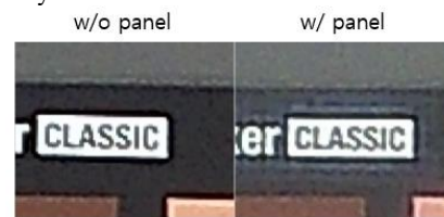
Figure 2. Image ghost on edge lines due to light diffraction
